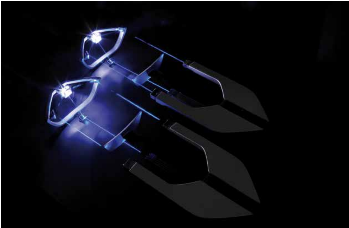
Picture 1: Experimental setup showing a white light produced by two Cerium(iii)-doped Yttrium Aluminum Garnet (Ce:YAG) phosphor-chips in a remote position that are excited by high-power multimode 450 nm laser diodes (over 1 W).
